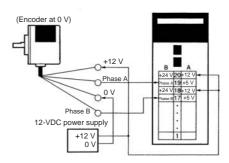
Note: Apply the following connections if the E6C3's 3 power supplies are 5 or 24 V.
